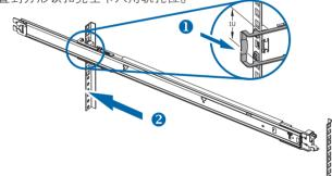
Pull up the latch release part on the front bracket. ②Push the rail into the rack until the square pins fully seat on the rack holes and the latch clicks into place. 将前固定件的释放件参照图中 ● 箭头拉开,再依图 ❷箭头将导轨推入,直到方形锁扣完全卡入角轨孔位。
