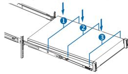
5 Press the side-release lock buttons on both rails and slide the system into the rack. 按压图中 ❶ 所示的导轨两侧卡扣,将服务器按照图中 ❷箭头所示的方向推入机柜。
