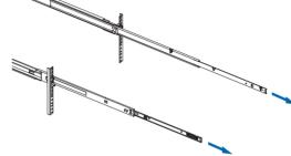
4 Align the rail stand off on each side of the system and lower them into the slots on the rail. Put the system downward until all the rail standoffs are seated in the slots.
