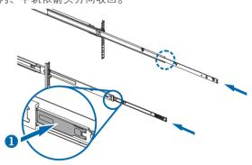
**4** Removing the rails as the same steps with installing. 依组装步骤拆卸导轨。
