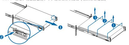
3 Press the side-release lock buttons on both rails and slide the rails into the rack.
