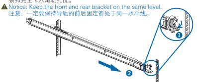
Repeat 1 and 2 steps to install the other side. And pull the inner rails out of the rack until they lock into place.
